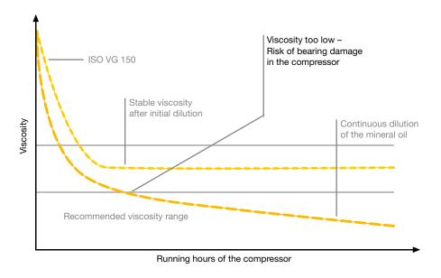
Mineral oil ISO VG 150 High viscosity decrease, viscosity not in line with specification
